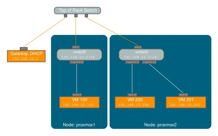
Bridges are like physical network switches implemented in software. All virtual guests can share a single bridge, or you can create multiple bridges to separate network domains. Each host can have up to 4094 bridges.
