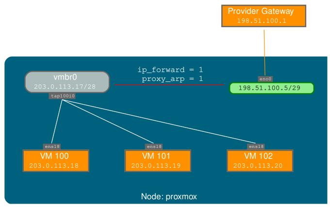
A common scenario is that you have a public IP (assume 198.51.100.5 for this example), and an additional IP block for your VMs (203.0.113.16/28). We recommend the following setup for such situations:
